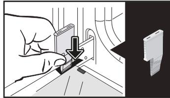
Remove the first clipped glass panel: Using the other wedge (or a screwdriver), press the slots **A** to unclip the glass.
