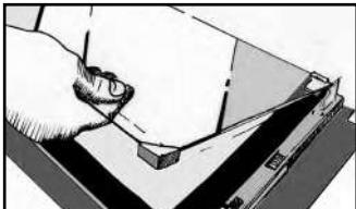
This assembly comprises 2 glass windows, the 1st of which has 2 rubber stops on the 2 front corners.
