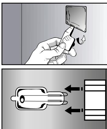
You can replace the bulb yourself. First disassemble the left-hand side shelf support.
