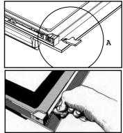
Lever the assembly to detach the frame and the glass.
