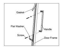
Remove the door gasket on the side you wish to install the handle - you can see two designated holes for handle installation.
