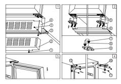
Remove the adjustable ventilation grille 0,2 by unscrewing the screws 0,1 and then remove the ventilation grille 0,4 by unscrewing the screws 0,3. (Fig. 1)
